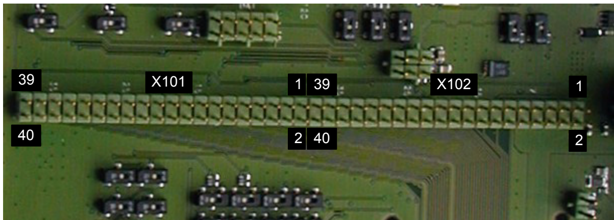
Figure 5: Overview of B2B connector pins and the corresponding test points
